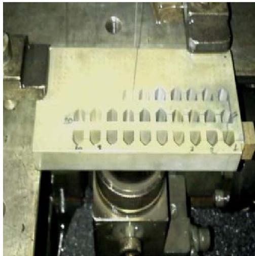
Fig. 1. Cavities produced in carbide block
