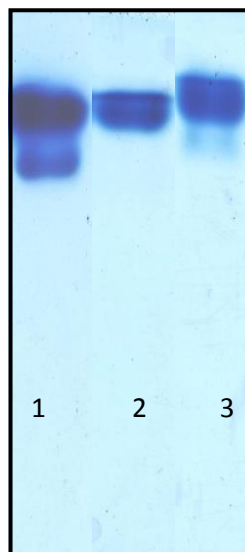
Fig. 3 Non-denaturing polyacrylamide gel electrophoresis using 15% acrylamide gel and glycine buffer, pH 4.3. Staining was by Coomassie Blue R-250.
