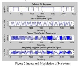
Figure 2 shows The 25 bits with 120 users is applied to input of wireless network. Based on the users available input bit streams are generated in the channel and carrier signal is allocated for each available user signal is modulated and phased shifted The spread signal
