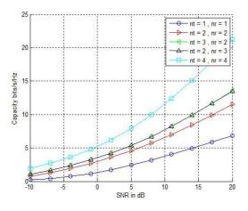
Figure 4 performance of MIMO wireless channel
