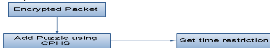
Fig 5. Cryptographic Puzzle Hiding Scheme
