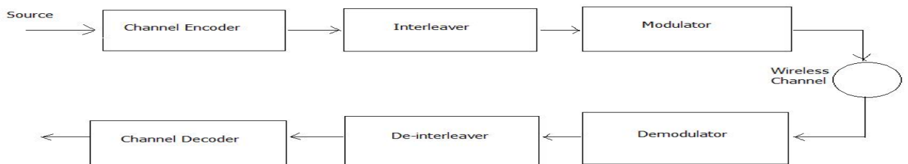
Fig 1. Generic Communication Classification Diagram
