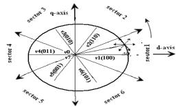
Fig.3 Relationship with voltage vectors and stator flux under DTC
