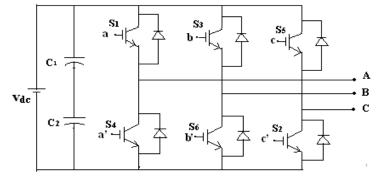
Fig.1 Schematic diagram of two level inverter
