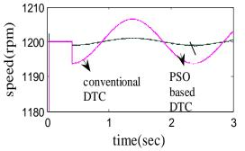
Fig.5 (b) Speed comparison with conventional and PSO based DTC
