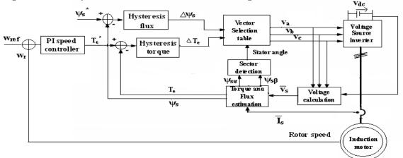
Fig.2 block diagram of IM drive under DTC
