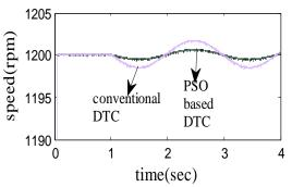
Fig. 7(b) Speed comparison with conventional and PSO based DTC
