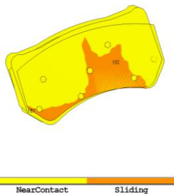
Fig.23: Contact status contour for 150RPS, cast iron material
