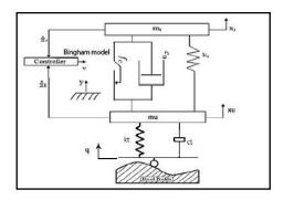
Figure 4: Quarter car vehicle with MR damper
