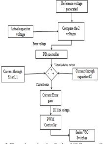
Fig 3 Flowchart for the Series VSC controller
