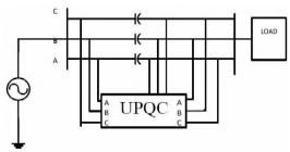
Fig 1 (b) - Single line diagram for the proposed system with crossconnected phaseat load side
