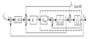
Fig 4 - Control Block diagram - Series VSC
