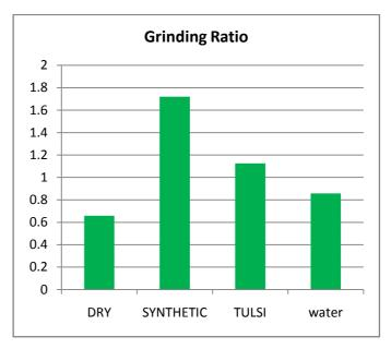
Fig. 5 Grinding ratio for synthetic coolant, dry, tulsi additive and water
