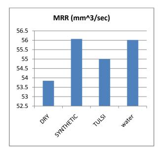
Fig. 3 Material removal rate for synthetic coolant, dry tulsi additive coolant and water
