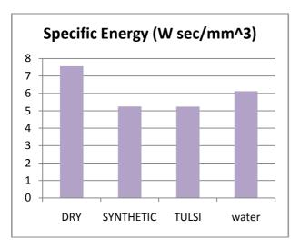
Fig.6. Specific energy for synthetic coolant, dry tulsi additive coolant and water
