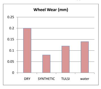
Fig. 4 Wheel wear for synthetic coolant, dry tulsi additive coolant and water
