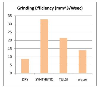
Fig.7. Grinding efficiency for synthetic coolant, dry tulsi additive coolant and water
