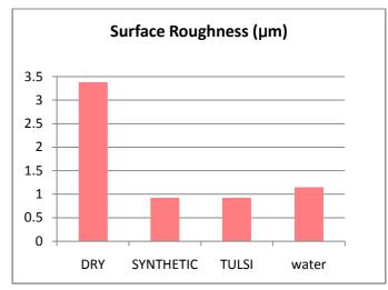
Fig-8 Surface Roughness for synthetic coolant, dry, tulsi additive coolant and water
