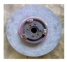
Fig. 2 Grinding wheel
