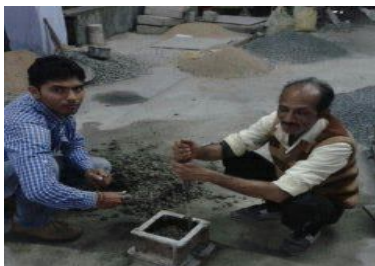
Figure (2.2) compaction of concrete manually.
