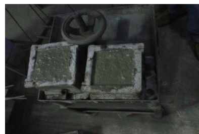
Figure(2.3) Compaction on vibrating table.
