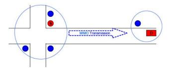
Fig.4. Cooperative MIMO transmission between infrastructure and vehicle
