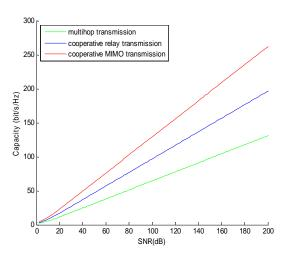
Fig 7. Channel capacity of Cooperative MIMO and Relay technique vs. multihop transmission with two transmission nodes,MQAM modulation over a Rayleigh channel
