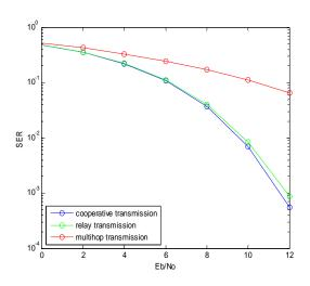
Fig .8.Interference of cooperative techniques vs multihop techniques.
