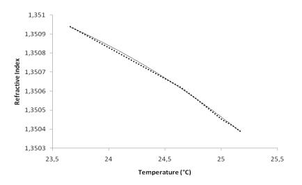
Figure 3. Variation of the refractive index of the juice as a function of temperature. Line solid: linear equations, Dot: experimental values.
