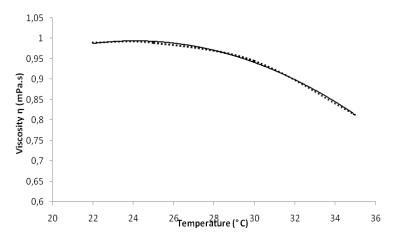
Figure 2. Variation of juice viscosity as a function of temperature. Line solid: linear equations, Dot: experimental values.
