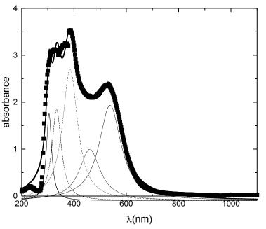
Figure 7. Curve fitting of the Ultraviolet-Visible Spectrum of thejuice of blueberries. experimental band; continuous lines. Cumulative Fit Peak; \_\_\_\_\_ - - -. ...... and - . - -. bands obtained in the fitting process: 304. 333. 345. 460 and 538 nm.
