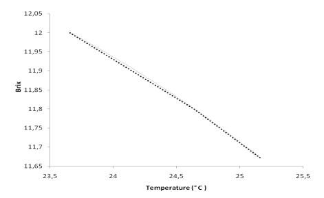
Figure 4. Brix variation of juice as a function of temperature. Line solid: linear equations, Dot: experimental values.
