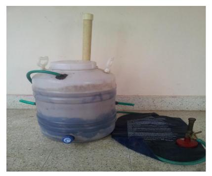
Fig. 2 Portable Biodigester
