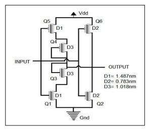
Fig. 3. Transistor level logic diagram of 6T STI
