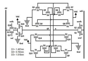
Fig. 5. Transistor level logic diagram of memory cell
