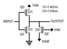
Fig. 2. Transistor level logic diagram of 3T STI
