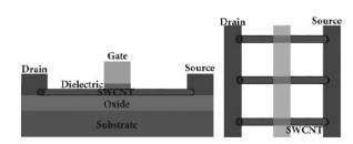
Fig.1. Schematic Diagram of CNTFET
