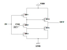
Fig. 3 Schematic of 5T-TSPC Clocked Latch
