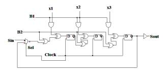
Fig. 2 Logic diagram of a BILBO
