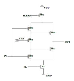
Fig .4 Schematic of 5T-TSPC (MTCMOS)
