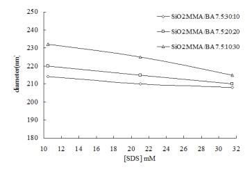
Figure 2. Initial monomer droplet sizes as a function of the concentration of SDS for silica-acrylate miniemulsion with various BA: MMA weight ratio.
