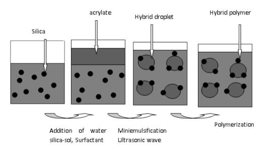
Figure 1. Principle of silica-sol-acrylate composite mini-emulsion polymerization.
