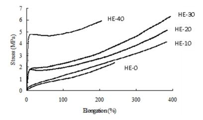
Figure 3. Strain-stress curves for silica-acrylate hybrid polymer with different amount of silica.
