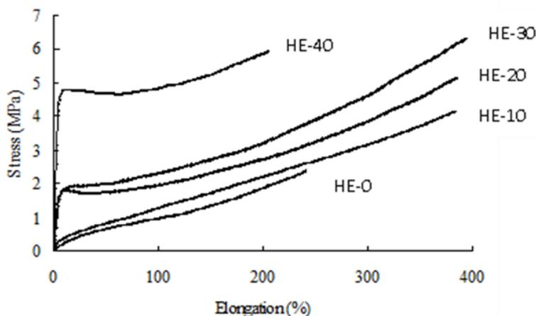
**Figure 3.** Strain-stress curves for silica-acrylate hybrid polymer with different amount of silica.
