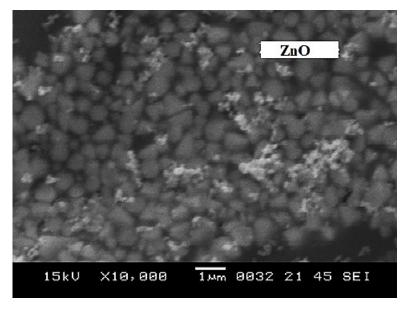
Figure 6. SEM of ZnO nanomaterial.
