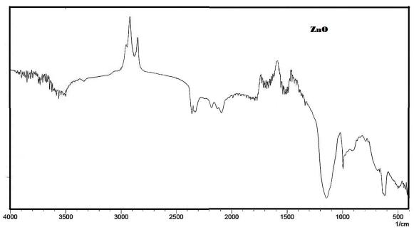
Figure 4. IR Spectra of ZnO.
