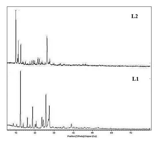
Figure 7. XRD of ZnO nanomaterial.
