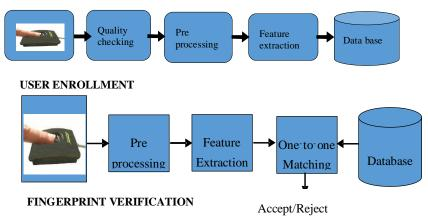
Fig. 2.2 User enrollment and fingerprint verification phases of the fingerprint-based user identification system.
