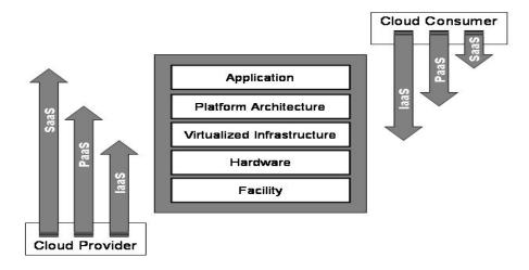
Figure 1: Differences in Scope and Control among Cloud Service Models
