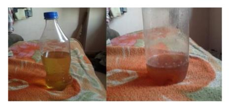
Figure 6. Separated biodiesel and glycerol from mixture.
