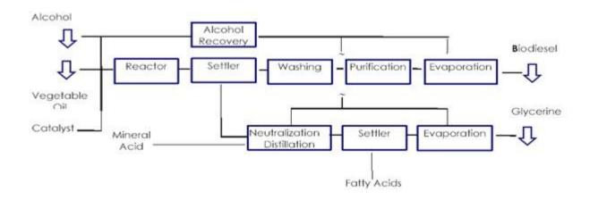
Figure 3. Flow sheet of biodiesel production [41].
