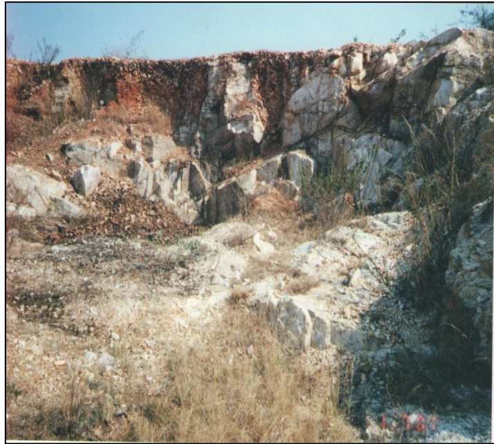
Photo 1: Quartz exposures occur as massive, semi-transparent and with three sets of joints.
