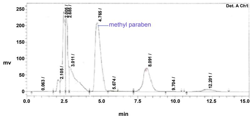
**Figure 4.** HPLC chromatogram of sample from batch 2. It shows the HPLC spectrum of sample (o/w skin cream). Where the identifying peak for methyl Paraben is come on retention time of 4.768.
