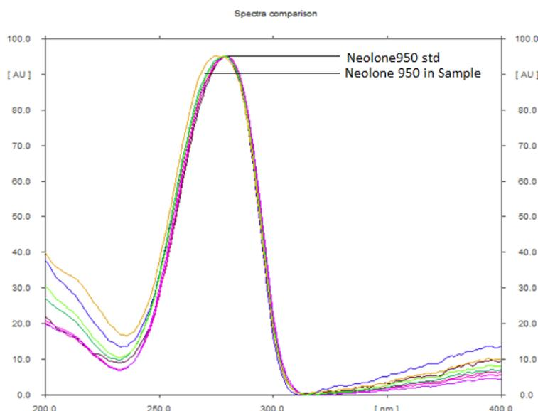
**Figure 16.** Spectrum scan of neolone 950. It shows the comparison between the standard and sample for spectrum matching of neolone 950 spectrum for sample and standard shows the super imposable image.
