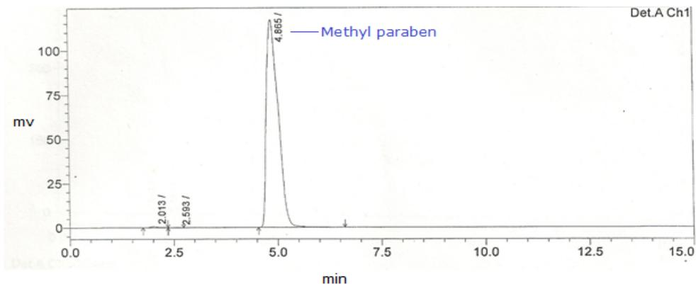
**Figure 1.** HPLC chromatogram of Standard Methyl Paraben.
