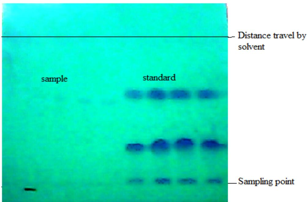
**Figure 13.** TLC plate of Neolone 950 (HPTLC). In this figure plate shown the standard and sample point for Neolone 950, With same Rf value. It helps to identify the presence of neolone 950 in sample.
