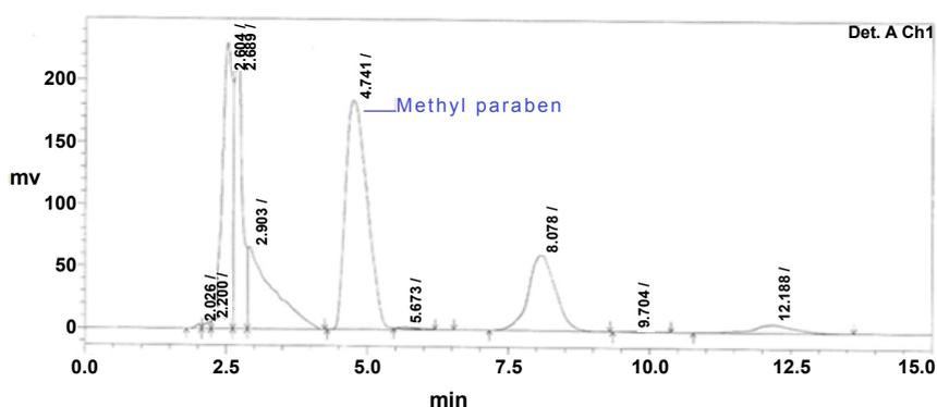
**Figure 5.** HPLC chromatogram of sample from batch 3. It shows the HPLC spectrum of sample (o/w skin cream) where the identifying peak for methyl Paraben is come on retention time of 4.741.
