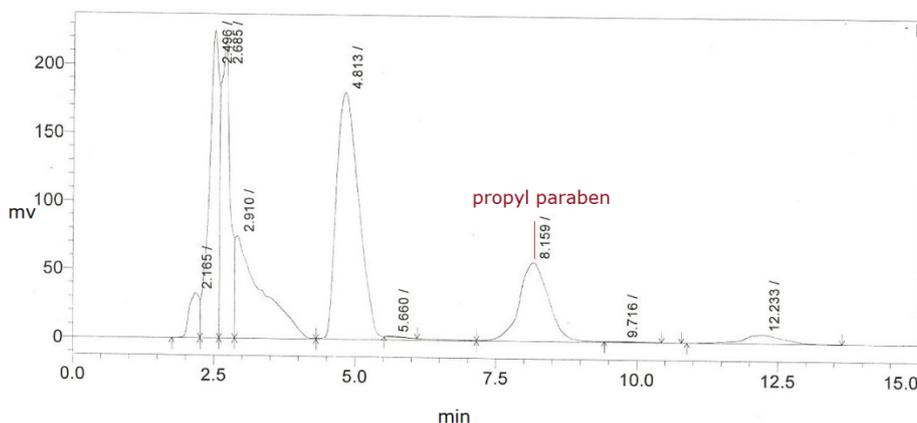
Figure 8. HPLC chromatogram of sample from batch 1. It shows the HPLC spectrum of sample (o/w skin cream) where the identifying peak for propyl Paraben is come on retention time of 8.159.
