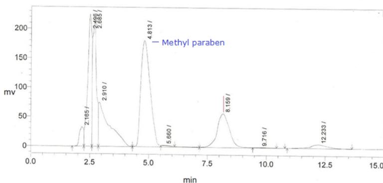
**Figure 3.** HPLC chromatogram of sample from batch 1. It shows the HPLC spectrum of sample (o/w skin cream). Where the identifying peak for methyl Paraben is come on retention time of 4.813.
