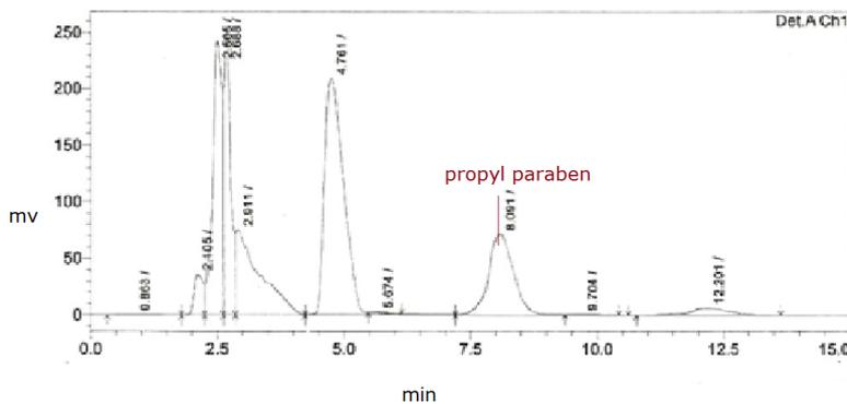
**Figure 9.** HPLC chromatogram of sample from batch 2. It shows the HPLC spectrum of sample (o/w skin cream) where the identifying peak for propyl Paraben is come on retention time of 8.091.
