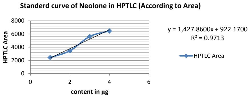
**Figure 11.** HPLC Standard curve of Neolone 950 (According to Area).
