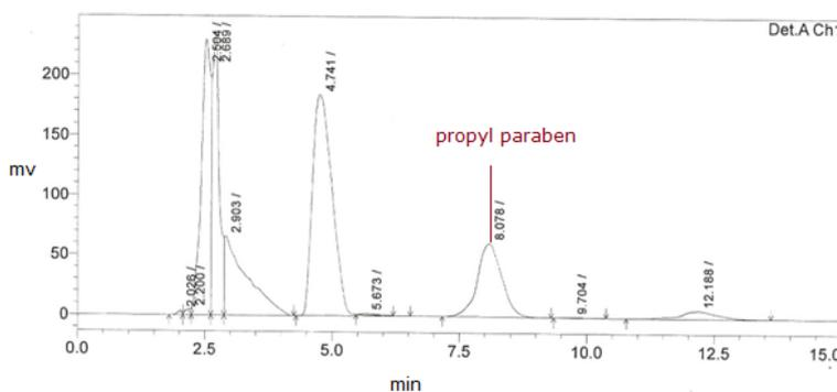
**Figure 10.** HPLC chromatogram of sample from batch 3. It shows the HPLC spectrum of sample (o/w skin cream) where the identifying peak for propyl Paraben is come on retention time of 8.078. Here the amount of propyl paraben in 3 different batch's sample are calculated by the regression equation of pure propyl paraben. Retention time of propyl paraben in sample is 8.1.
