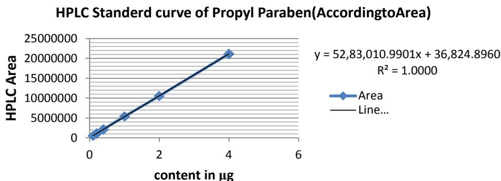
Figure 7. HPLC Standard curve of Propyl Paraben (According to Area). Regression via Area  $y = 52,83,010.9901x + 36,824.8960$ .
