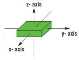
Fig.3. Three-axis direction of MEMS accelerometer
