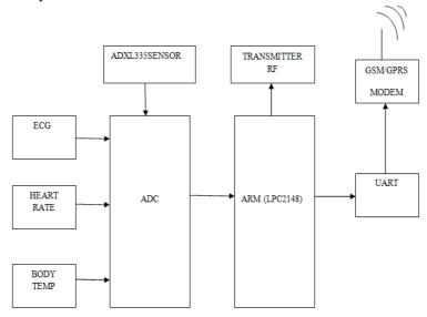
Fig.1. Block Diagram for proposed system
