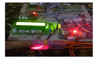
The GSM (Global System for Mobile communication) modem transmits these events to the mobile phones of care takers/ relatives of the fallen human as a message shown as yellow box. This alert message helps to provide immediate assistance and treatment. Temperature, heart rate is displayed in the below output window.
