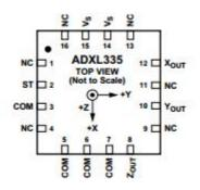
Fig.4. ADXL 335 Pin Configuration.
