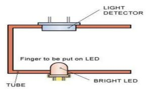
Fig.5. Sensor Construction.
