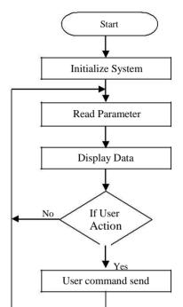
Fig. 4 Flow chart for receiving station of grain storage system
