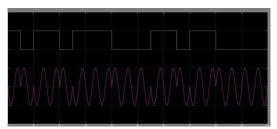
Figure 7: BPSK modulation
