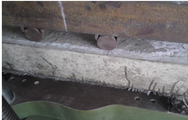
Figure 4. Beam with glass fibre wrapped in tensile zone
