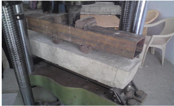
Figure 2. Experimental Setup - Beam with two point loading
