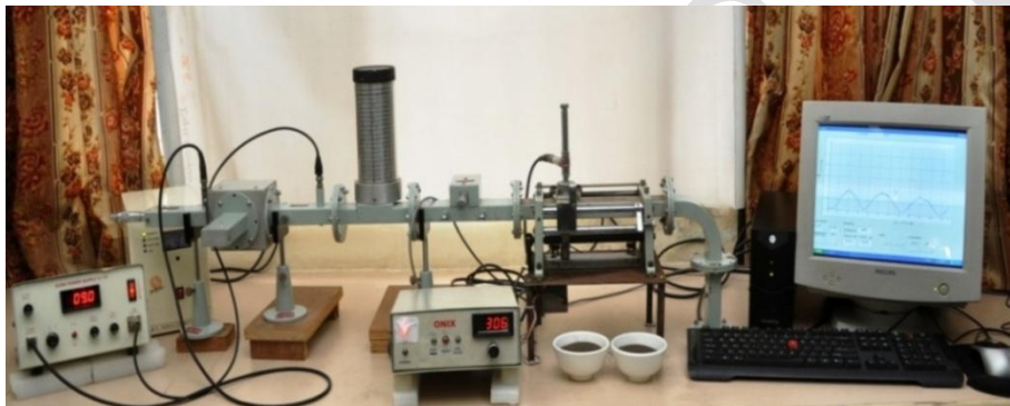
Fig. 1. C-Band microwave setup for measurement of dielectric constant of Soils
