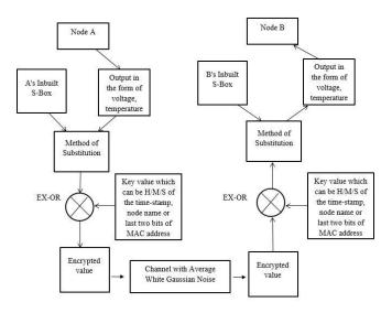
Figure 4: High level Block Diagram of the prosposed encryption and decryption process.
