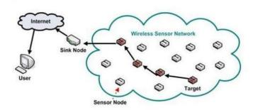
Figure 1: Wireless Sensor Network Architecture.
