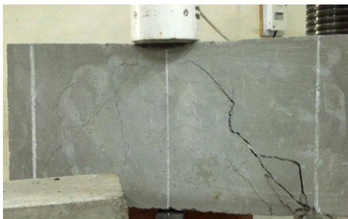
Fig. 2 Cracks developed on hexagonal mesh
