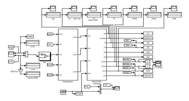
Fig.8 Simulation Block For DTC With PID System
