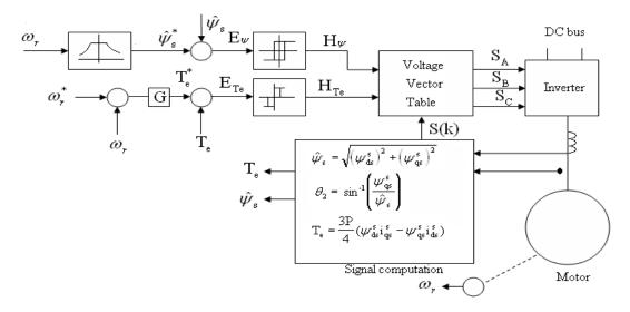
Fig.6 Direct Torque and Flux Control Block Diagram
