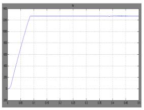
Fig.13 Speed of the Induction Motor With ANN Based SVM
