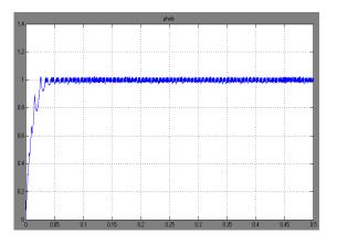
Fig.14 Stator Flux Magnitude conventional DTC
