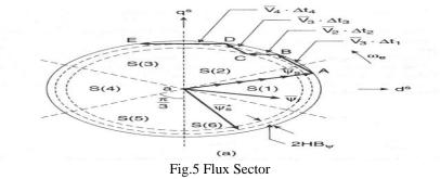
The voltage vector receives the input signals  $H_{\Psi}$   $H_{Te}$  and S(k) generates the appropriate control voltage vector (switching states) for the inverter by lookup table, which is shown in Table-1 (the vector sign is deleted). The inverter voltage vector (six active and two zero states) and a typical  $\Psi_s$  are shown in Figure 5. Neglecting the stator resistance of the machine.
