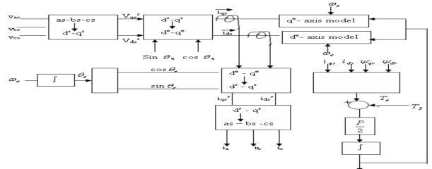
Fig.4 Synchronously Rotating Frame Machine Models with Input Voltage and Output Current Transformations
