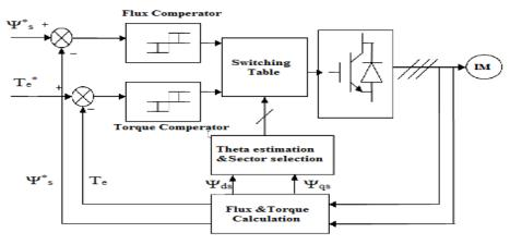
Fig. 1 Basic Direct Torque Control Scheme for AC Motor Drives
