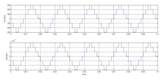
Fig. 8 Simulation result of seven level inverter
