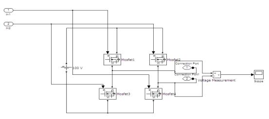
Fig. 3 Bridge circuit for three level inverter
