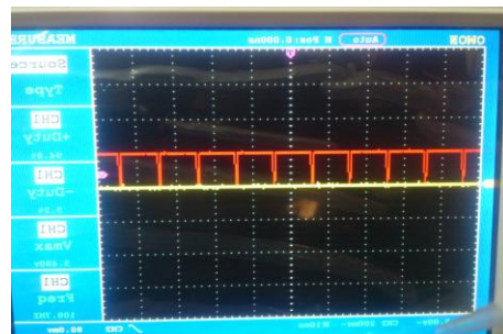
Fig 23: Zero crossing of Voltage
