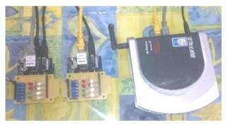
Fig. 7: 2 RTU's with Wireless High Power Module [1]
