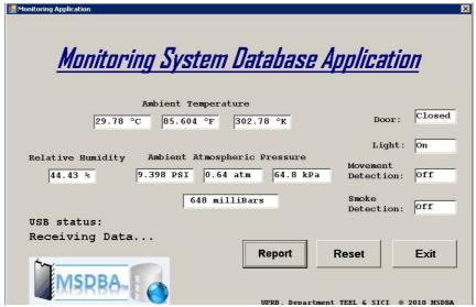
Figure 9. PC client interface program to monitor physical variables in a room.
