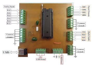
Figure 11. Prototype circuit board of the data acquisition module
