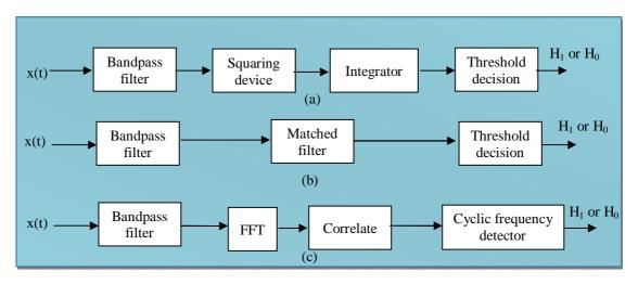
Fig 1: Block diagrams for narrowband spectrum sensing techniques: a) energy detection; b) matched filtering; c) cyclostationary feature detection
