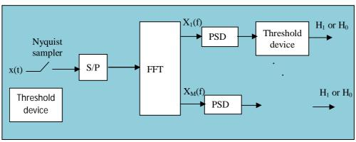
Fig 2: block diagram of Nyquist wideband spectrum sensing techniques
