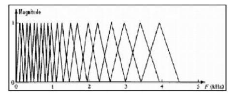
Fig-2 Mel filter bank with overlapping filters
