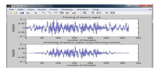
Fig-5 Framing and windowing of speech signal
