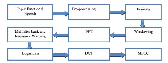
Fig-1 Block Diagram for MFCC feature extraction
