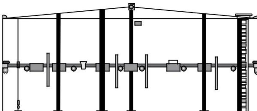
Figure 3. Internal floating roof tank.
