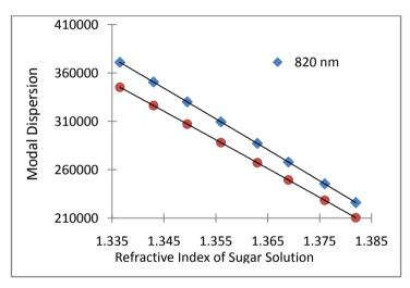
Fig(10):The relation showing variation of Modal Dispersion with refractive index at operating wavelengths 820nm and 850nm for guiding liquid of sugar solution.
