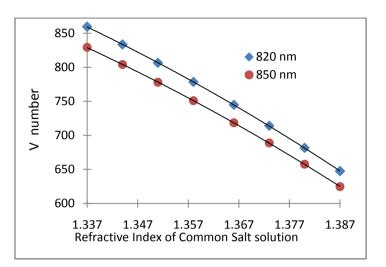
Fig(7): The relation showing variation of V-number with refractive index at operating wavelengths 820nm and 850nm for guiding liquid of common salt solution
