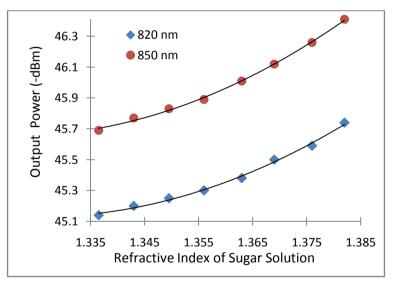
Fig(4): Graph showing the relationship between refractive index and output power at operating wavelengths 820nm and 850nm for guiding liquid of Sugar solution
