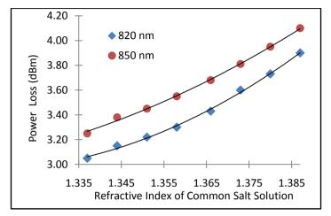
Fig(5): Graph showing the relationship between refractive index and power loss atoperating wavelengths 820nm and 850nm for guiding liquid of common salt solution
