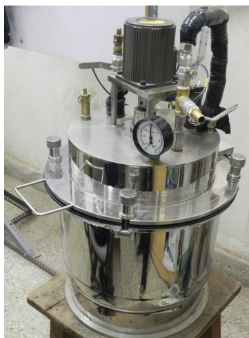
Fig.2 photograph of the cryotreatment unit
