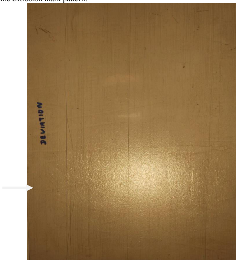
Fig. 10. Transparent bag showing a deviation (9.1.cm long) of an extrusion line observed in a plastic bag.
