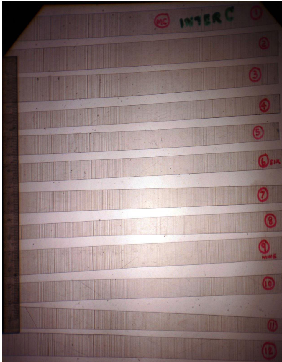
Fig. 9. Inter-batch stability of extrusion mark pattern in the samples of plastics from the same known machine No.2 collected in 12 months (sample nos. 2/1 to 2/12).
