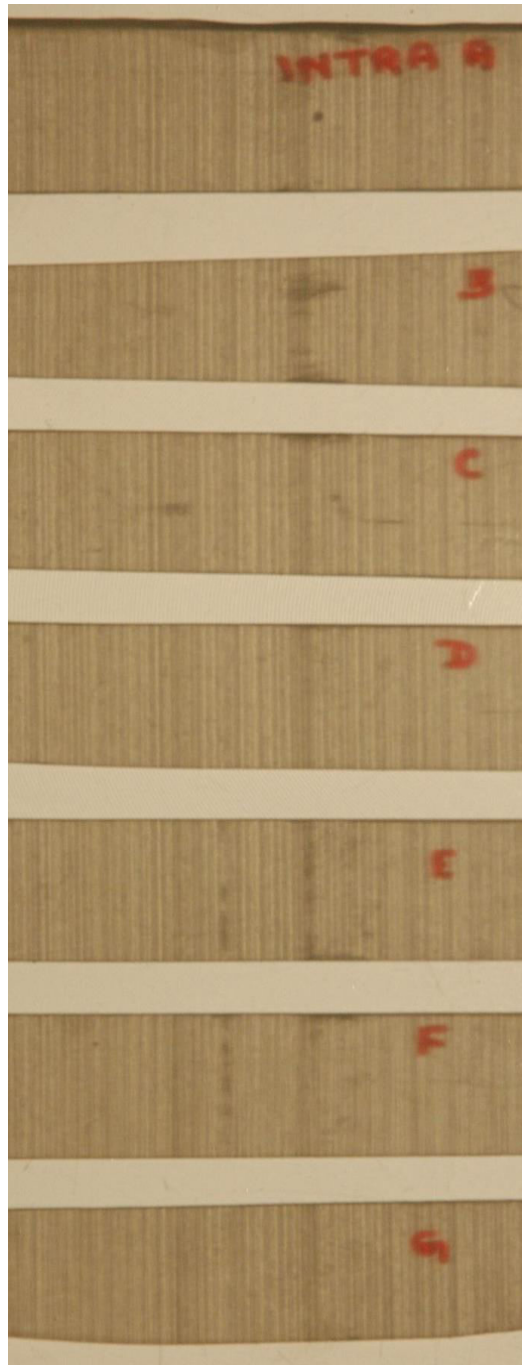
Fig. 6. Intra batch stability of extrusion mark pattern in the different areas in the length of a blown plastic tube manufactured on a known date from a known machine
