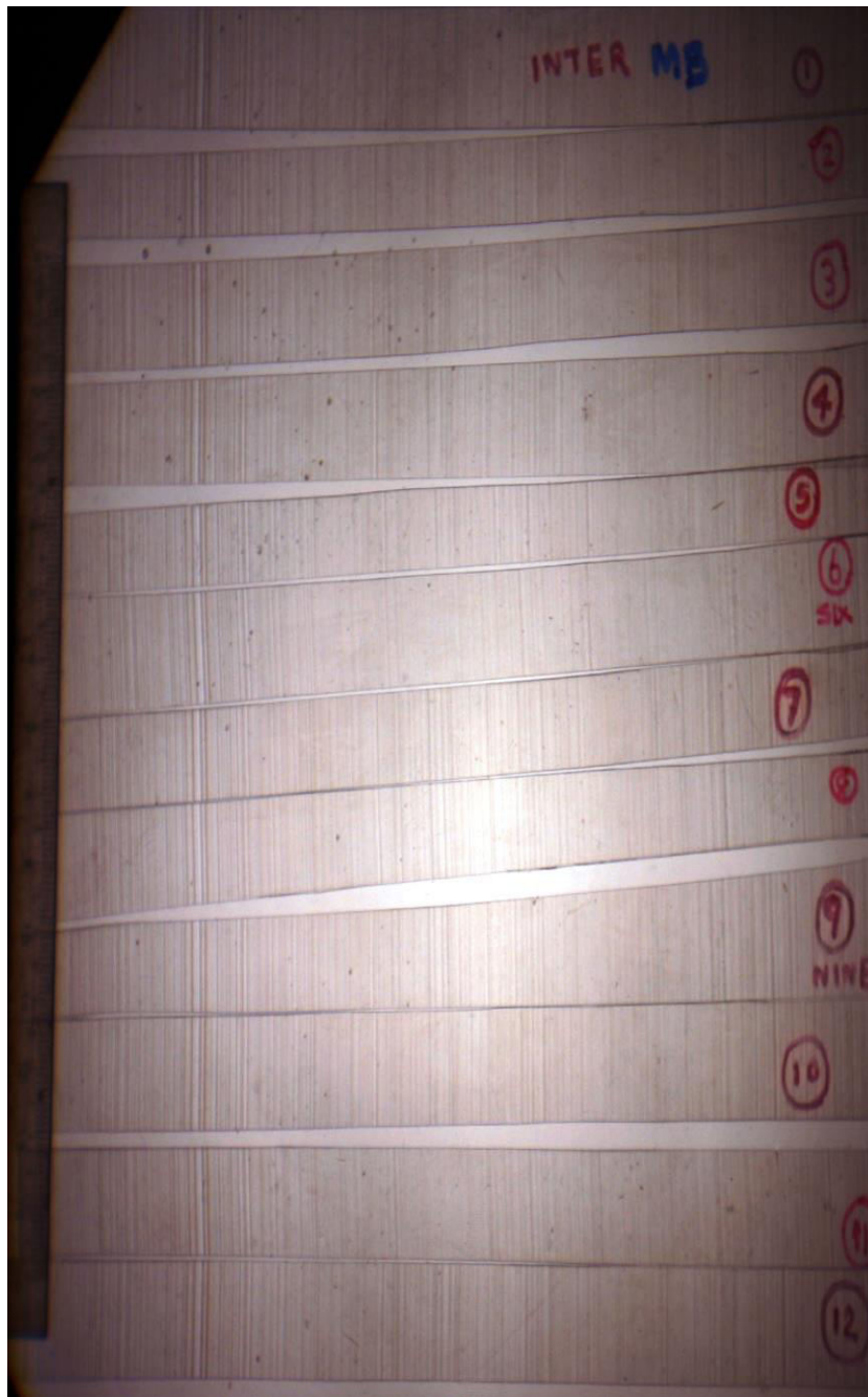
Fig. 8. Inter-batch stability of extrusion mark pattern in the samples of transparent plastics from the same known machine No.1 collected in 12 months (sample nos. 1/1 to 1/12).
