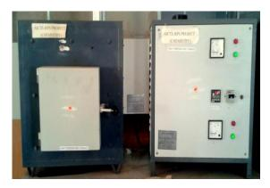
Fig.2: Diagram shows the high temperature furnace. As the paste which is applied over the material is in wet condition, it has to be dried off before it is taken for Induction boriding.
