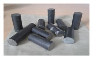
Fig. 1: high speed steel of M2 grade.
