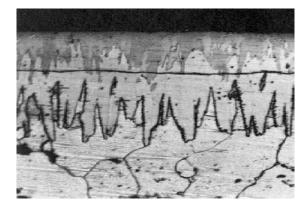
Fig. 7: Sawtooth structure
