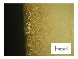
Diagram A & B clearly shows the formation of borides over the high speed steel. We can also concludes the diffusion of Boron instead of coating.
