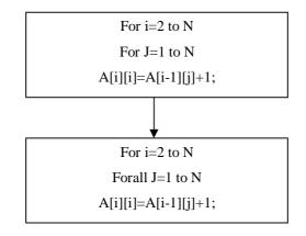
Fig. 4: Loop Parallelization
