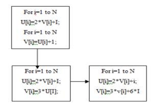
Fig.1: Loop Fusion
