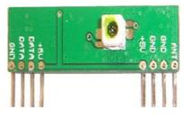
Fig. 4. RF Receiver STT-433MHZ.
