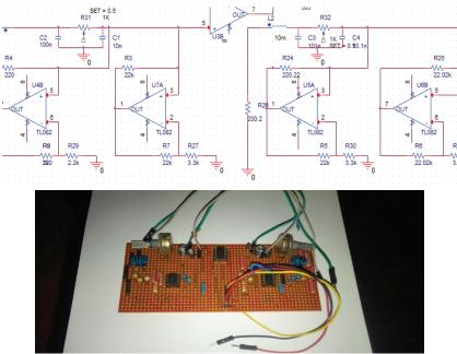
Figure 8. The Chua circuit implementation of the design.
