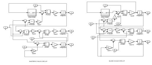
Figure 6. Model for master and slave Chua's oscillator.
