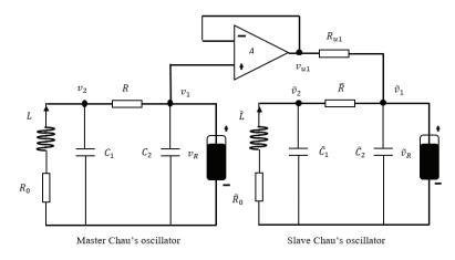
Figure 5. Master/slave Chau's oscillators.
