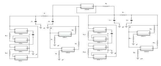
Figure 4. Current conveyors based realization of two Chua's oscillator.
