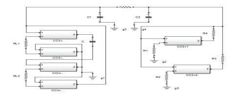
Figure 3. Current conveyors based realization of Chua's oscillator.
