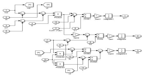
Figure 7. Model for master/slave Chua's oscillator.
