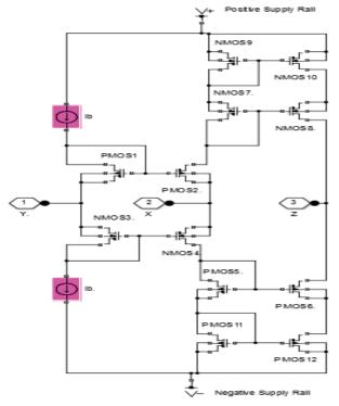
Figure 9. CMOS realization of the CCII+ used in simulations.
