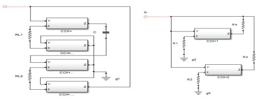
Figure 1. (a): simulated inductance in CCII+; (b):chua's diode in CCII+.
