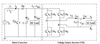
Fig 4: Traditional two-stage dc-to-ac conversion system: Boost converter cascaded with a VSI.
