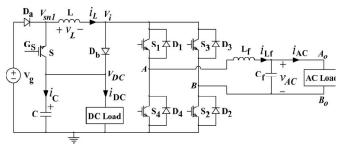
Fig 2: Circuit diagram of SBI supplying both dc and ac loads.
