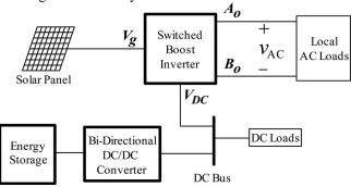
Fig 1:structure of the proposed DC grid.
