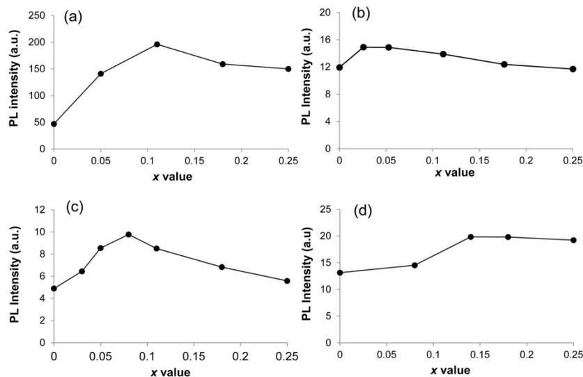
**Figure 4.** Changes of PL intensities with x-values (concentrations of Ti) of (a)  $\text{Li}_{1+x}\text{Ta}_{1-x}\text{Ti}_x\text{O}_3:\text{Eu}^{3+}$ , (b)  $\text{Li}_{1+x}(\text{Ta}_{0.2}\text{Nb}_{0.8})_{1-x}\text{Ti}_x\text{O}_3:\text{Er}^{3+}$ , (c)  $\text{Li}_{1+x}(\text{Ta}_{0.4}\text{Nb}_{0.6})_{1-x}\text{Ti}_x\text{O}_3:\text{Tm}^{3+}$ , and (d)  $\text{Li}_{1+x}(\text{Ta}_{0.6}\text{Nb}_{0.4})_{1-x}\text{Ti}_x\text{O}_3:\text{Dy}^{3+}$ .
