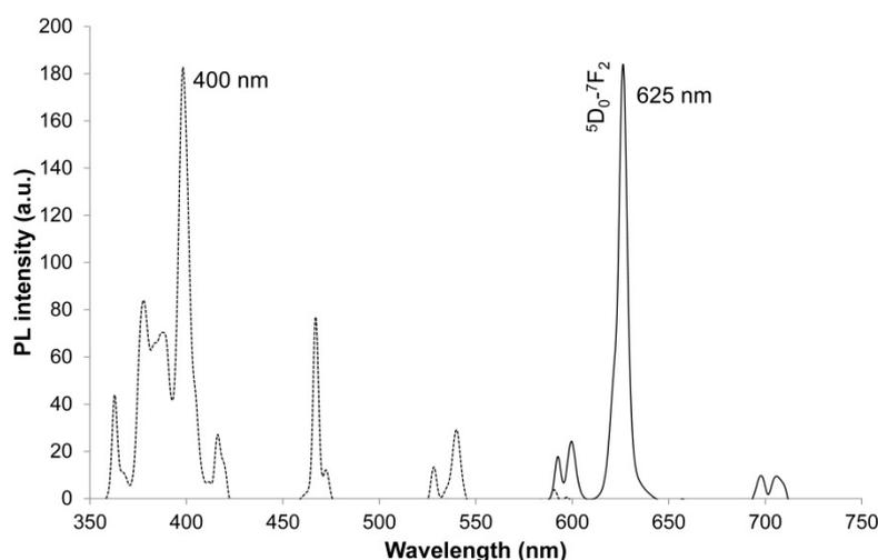
**Figure 5.** Excitation and emission spectra of  $\text{Li}_{1.11}\text{Ta}_{0.89}\text{Ti}_{0.11}\text{O}_3:\text{Eu}^{3+},\text{Sm}^{3+}$ .
