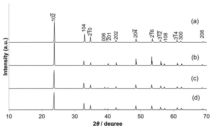
**Figure 8.** XRD patterns of (a)  $\text{Li}_{1.11}\text{Ta}_{0.89}\text{Ti}_{0.11}\text{O}_3:\text{Eu}^{3+},\text{Sm}^{3+}$ , (b)  $\text{Li}_{1.03}(\text{Ta}_{0.2}\text{Nb}_{0.8})_{0.97}\text{Ti}_{0.03}\text{O}_3:\text{Er}^{3+}$ , (c)  $\text{Li}_{1.08}(\text{Ta}_{0.4}\text{Nb}_{0.6})_{0.92}\text{Ti}_{0.08}\text{O}_3:\text{Tm}^{3+}$ , and (d)  $\text{Li}_{1.14}(\text{Ta}_{0.6}\text{Nb}_{0.4})_{0.86}\text{Ti}_{0.14}\text{O}_3:\text{Dy}^{3+}$ .
