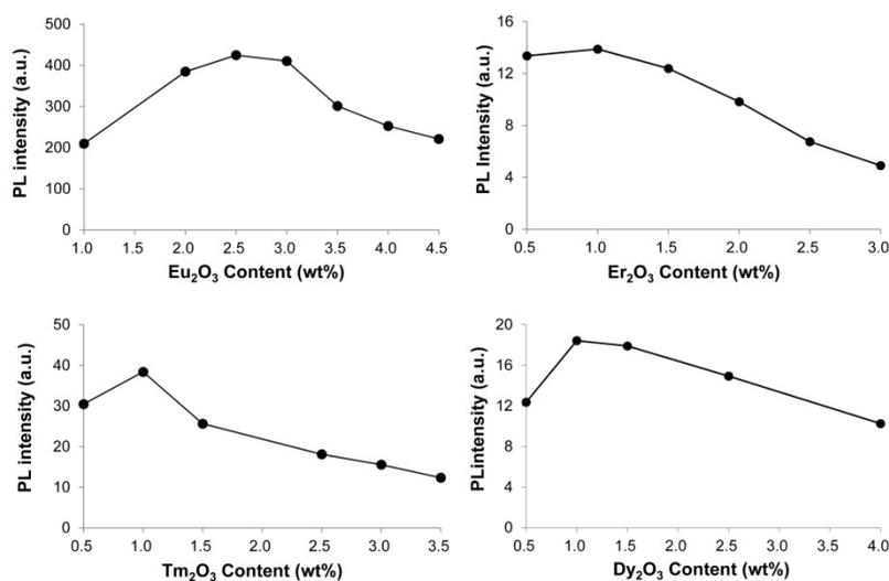
**Figure 3.** Changes of PL intensities with  $\text{RE}_2\text{O}_3$  concentrations of  $\text{Li}_{1.11}\text{Ta}_{0.89}\text{Ti}_{0.11}\text{O}_3:\text{RE}^{3+}$ . Phosphors activated with (a)  $\text{Eu}^{3+}$ , (b)  $\text{Er}^{3+}$ , (c)  $\text{Tm}^{3+}$ , and (d)  $\text{Dy}^{3+}$ .
