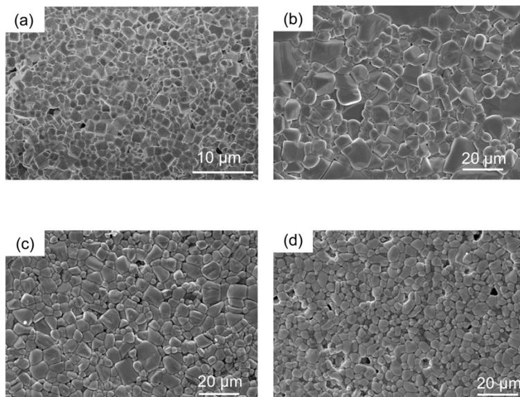
**Figure 7.** SEM images of (a)  $\text{Li}_{1.11}\text{Ta}_{0.89}\text{Ti}_{0.11}\text{O}_3:\text{Eu}^{3+},\text{Sm}^{3+}$ , (b)  $\text{Li}_{1.03}(\text{Ta}_{0.2}\text{Nb}_{0.8})_{0.97}\text{Ti}_{0.03}\text{O}_3:\text{Er}^{3+}$ , (c)  $\text{Li}_{1.08}(\text{Ta}_{0.4}\text{Nb}_{0.6})_{0.92}\text{Ti}_{0.08}\text{O}_3:\text{Tm}^{3+}$ , and (d)  $\text{Li}_{1.14}(\text{Ta}_{0.6}\text{Nb}_{0.4})_{0.86}\text{Ti}_{0.14}\text{O}_3:\text{Dy}^{3+}$ .
