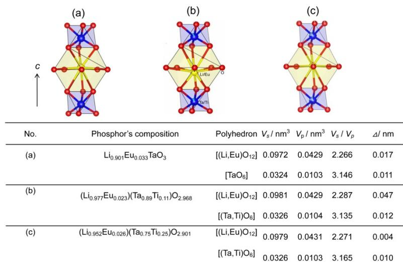
**Figure 9.** Structural models viewed along  $^{[11]}$  and structural data of  $\text{Li}_{0.901}\text{Eu}_{0.033}\text{TaO}_3$ ,  $(\text{Li}_{0.977}\text{Eu}_{0.023})(\text{Ta}_{0.89}\text{Ti}_{0.11})\text{O}_{2.968}$  and  $(\text{Li}_{0.952}\text{Eu}_{0.026})(\text{Ta}_{0.75}\text{Ti}_{0.25})\text{O}_{2.901}$  phosphors.
