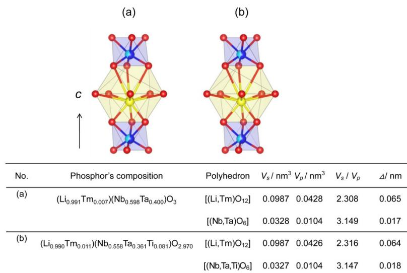
**Figure 10.** Structural models viewed along  $^{[11]}$  and structural data of  $(\text{Li}_{0.991}\text{Tm}_{0.007})(\text{Nb}_{0.598}\text{Ta}_{0.400})\text{O}_3$  and  $(\text{Li}_{0.990}\text{Tm}_{0.011})(\text{Ta}_{0.361}\text{Nb}_{0.558}\text{Ti}_{0.081})\text{O}_{2.970}$  phosphors.
