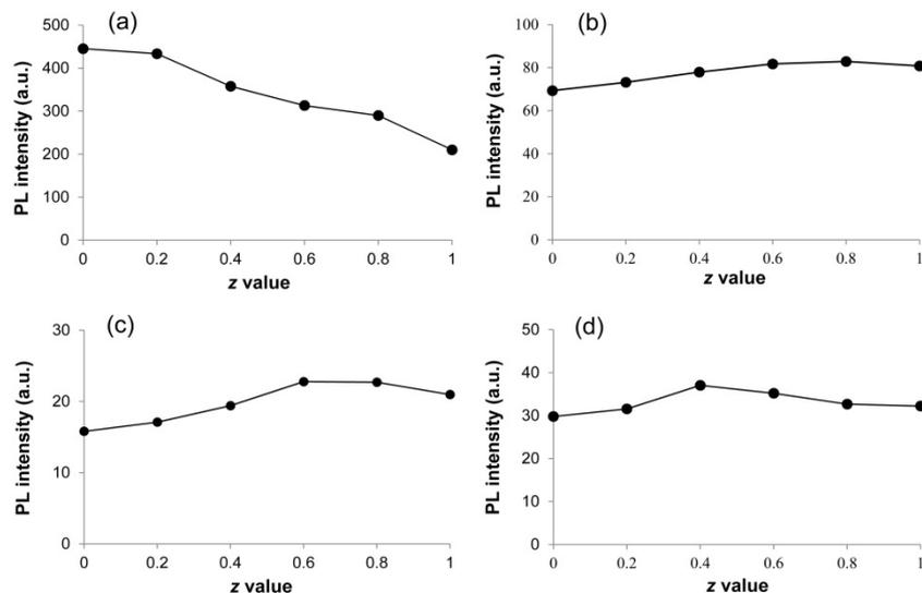
**Figure 2.** Changes of PL intensities with z values of  $\text{Li}_{1.11}(\text{Ta}_{1-z}\text{Nb}_z)_{0.89}\text{Ti}_{0.11}:\text{RE}^{3+}$  ( $\text{RE}_2\text{O}_3$ : 2.5 wt%). Phosphors activated with (a)  $\text{Eu}^{3+}$ , (b)  $\text{Er}^{3+}$ , (c)  $\text{Tm}^{3+}$ , and (d)  $\text{Dy}^{3+}$ .
