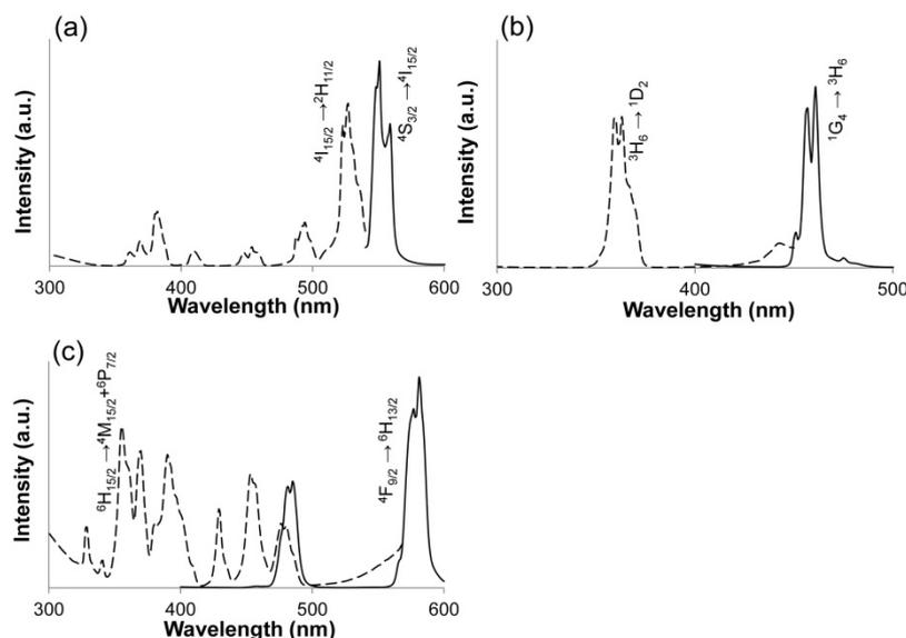
**Figure 6.** Emission and excitation spectra of (a)  $\text{Li}_{1.03}(\text{Ta}_{0.2}\text{Nb}_{0.8})_{0.97}\text{Ti}_{0.03}\text{O}_3:\text{Er}^{3+}$ , (b)  $\text{Li}_{1.08}(\text{Ta}_{0.4}\text{Nb}_{0.6})_{0.92}\text{Ti}_{0.08}\text{O}_3:\text{Tm}^{3+}$ , and (c)  $\text{Li}_{1.14}(\text{Ta}_{0.6}\text{Nb}_{0.4})_{0.86}\text{Ti}_{0.14}\text{O}_3:\text{Dy}^{3+}$ .
