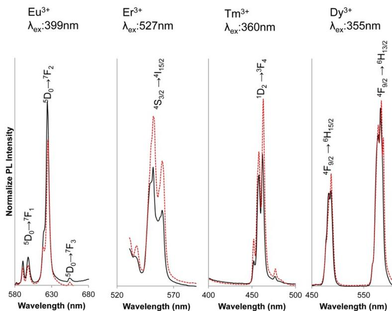
**Figure 1.** Emission spectra of  $\text{Li}_{1.11}(\text{Ta}/\text{Nb})_{0.89}\text{Ti}_{0.11}\text{O}_3:\text{RE}^{3+}$ . Dotted line is for LNT: $\text{RE}^{3+}$  and solid line is for LTT: $\text{RE}^{3+}$  [13].
