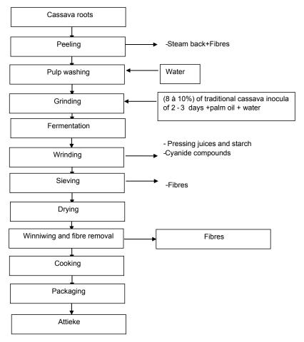
Figure 2. Process of attieke production in Cote d'Ivoire.
