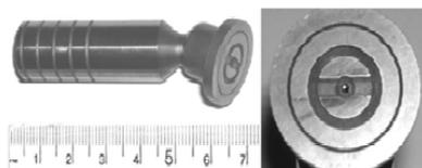
Figure 4. Piston and slipper assembly.
