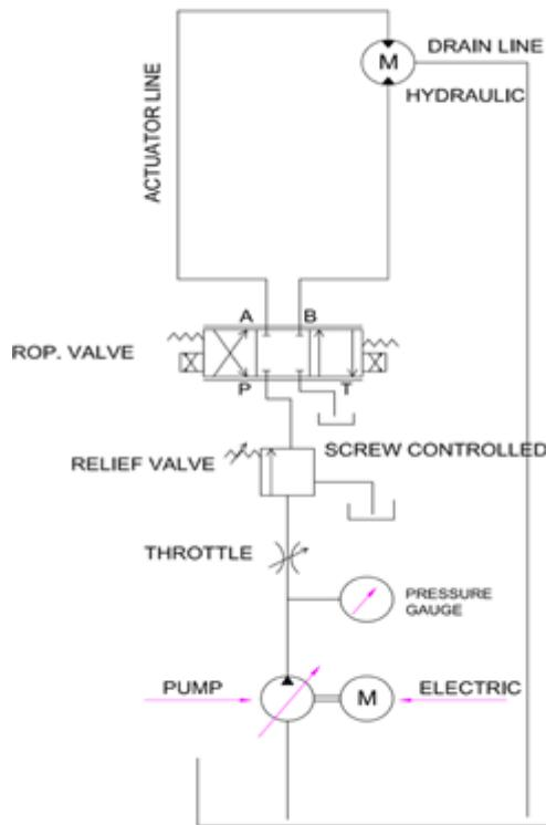
Figure 8. Simple hydraulic circuit.
