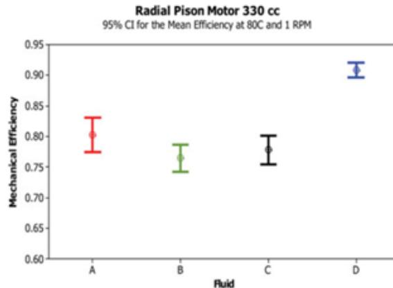
Figure 10. 1 rpm efficiency results for 330 cc radial piston motor at 80 degrees centigrade.
