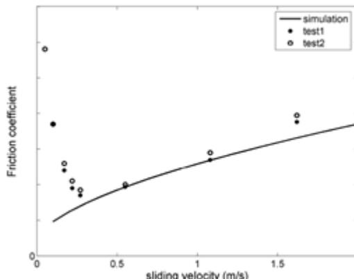
Figure 3. The friction coefficient in the roller piston interface, measured in the piston test rig.
