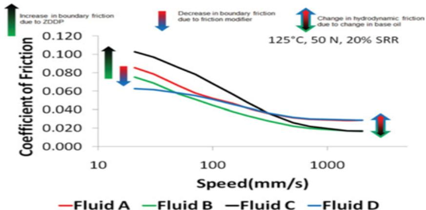
Figure 9. Stribeck curves of the fluids tested.
