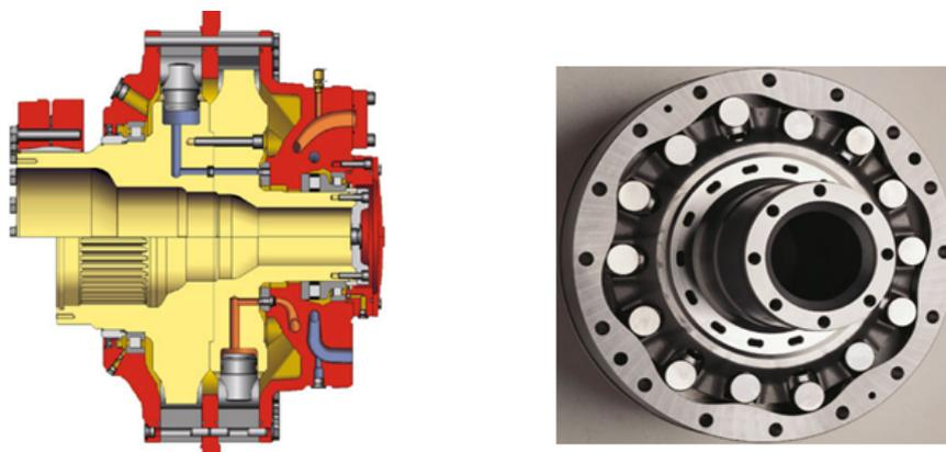
Figure 2. Radial piston motor (schematic (left) and real-life cross).
