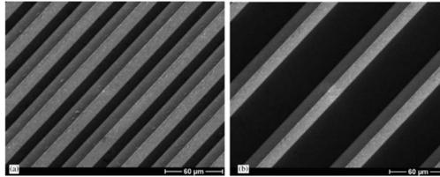
Figure 5. (a): Diamond embossing tool surfaces with ridge spacing of 30 micrometres; (b): 60 micrometres.
