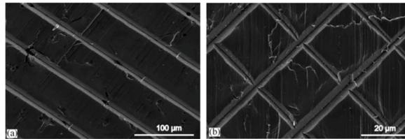
Figure 6. Textured piston sample before testing (a): parallel groove; (b): mesh pattern groove.
