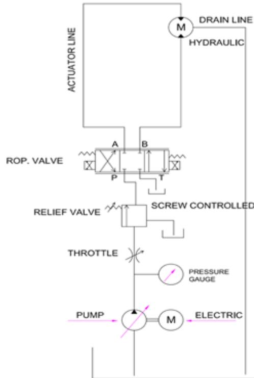
Figure 8. Simple hydraulic circuit.
