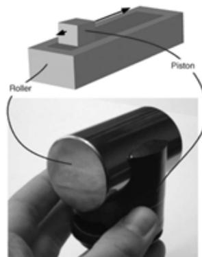
Figure 7. Roller piston assembly.
