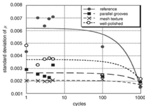
Figure 11. Friction fluctuation as a function of number of strokes.
