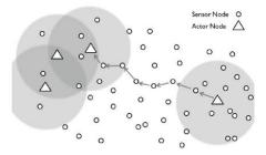
Fig.3 An isolated actor finding a path to other actors through sensor nodes
