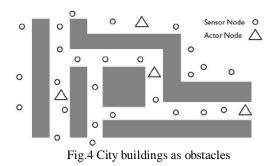
A network model for the disconnected IAN is presented. The model is as follows. A WSAN is represented as an undirected graph G = (V,E). V = S UA where S denotes a sensor set and A denotes an actor set.  $E = (S \times S) U(S \times A)$  denotes an edge set that includes sensor-sensor and sensor-actor connections. A
