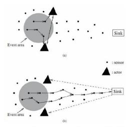
Fig. 1. (a) Automated and (b) semi-automated architecture of WSANs [3]
